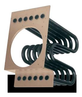
One standard feature of all Lennox unit heaters and duct furnaces is the tubular heat exchanger, designed to enhance performance and reliability. The exchanger's curved design provides excellent heat transfer by completely exposing the heating surface to the air stream. Rounded surfaces minimize air resistance and even heating is allowed across all surfaces, reducing stress on the heat exchanger.
